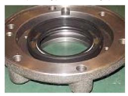
b) Place a disk-like inserting jig (which is slightly larger than the oil seal) onto the oil seal. While holding the jig by hand, lightly hit it in the top, bottom, right and left with a hammer to insert the oil seal gradually (see the following picture to the right).
