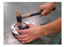
c) As soon as the motor oil seal is inserted in the motor oil retainer [618], the mounting is complete. For the compressor oil seal, after inserting the compressor oil seal retainer [26], install the oil seal gland [32-1]. Mount the oil seal gland and tighten it with four bolts [32-2] (following picture to the right).
