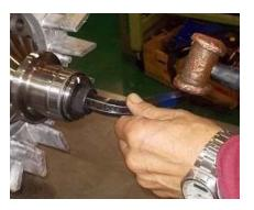
e) If the motor bearing [613] is replaced, fix the inner bearing race on the motor rotor by shrink-fitting. Heat up the inner bearing race to a temperature of 80 to 100°C by using a bearing heater or the like to fix it on the motor rotor shaft, and attach the motor bearing snap ring B [613-2].
