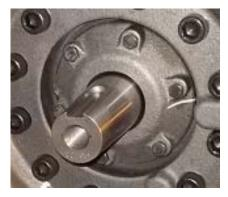
When replacement of the oil seal is required, remove the four bolts [32-2] that are tightening the compressor oils seal gland [32-1] (following picture to the left), and take off the oil seal gland.
