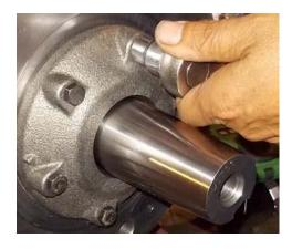
c) While holding the oil seal retainer, screw in the bolts [28] (above picture), and tighten them with the specified torque.
