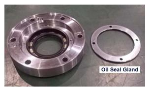
c) To remove the compressor oil seal, while allowing the edge of a flat blade screwdriver to hit on the slightly exposed part of the inner circumference of the oil seal through the shaft hole of the oil seal retainer, hit the head of the screwdriver with a hammer to push out the oil seal (picture to the right). While changing the hitting position of the screwdriver little by little, gradually push it out.
