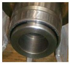
When replacing the bearing, remove the snap ring B [613-2] that is fit in front for retaining the motor bearing, and heat up the outer circumference of the inner bearing race with a gas torch or the like to remove it.
