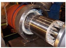
Motor Rotor Fin and Stator Winding
